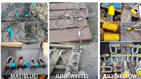
Lifting Tools Inspection & Colour Coding (Monthly)
